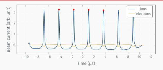
$\cdot$  electron time axis shifted by measured  $\Delta$  in propagation delay: 286 ns
