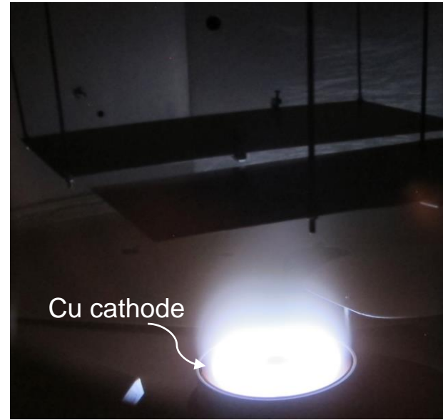
Cu coating by planar magnetron sputtering
