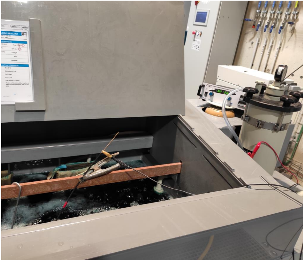
Acidic copper sulphate with brightener bath
